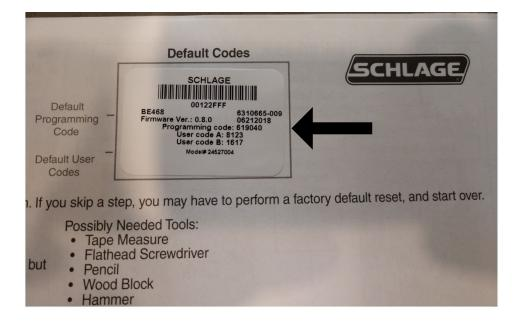
Additionally, if the sticker cannot be located, the codes are on the back of the interior assembly. By removing the two screws that fasten the lock hardware to the door you will be able to obtain the codes.
